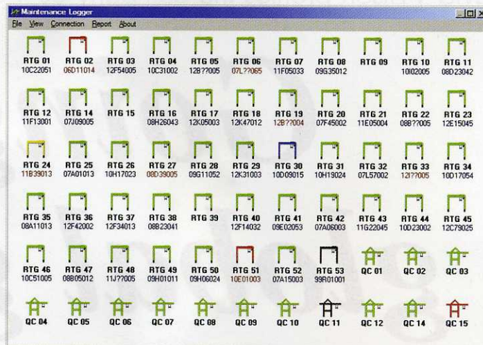
The ITS software includes GPS and container move identification systems that allow units to be tracked in real time
